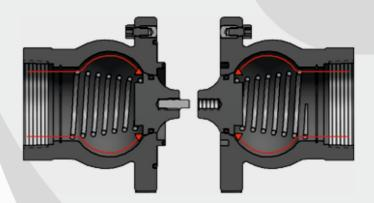
Flow position under normal operation: The coupling consists of two halves, each with a valve (piston) which is open.
